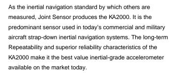
As with the entire family of accelerometers, the KA2000 has an amorphous quartz proof-mass structure which provides excellent bias, scale factor, and axis alignment Repeatability.
